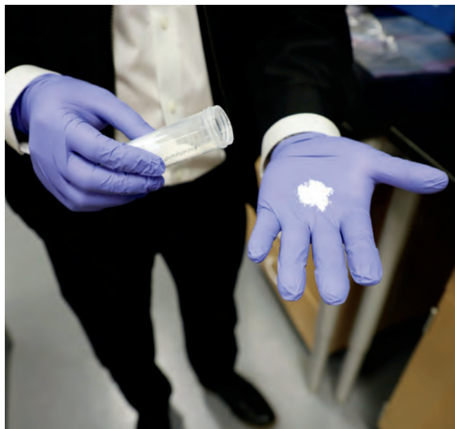
The high-performance powder is based on the polyamic acid (PAA) polymer, which has a low melting point.
